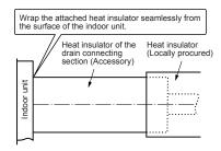
Direct the slits and seams of the heat insulator upward to avoid water leakage.
