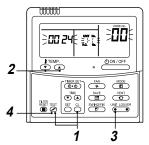
Push 🖰 and 🐺 buttons simultaneously for at least 4 seconds to call the service monitor mode.
