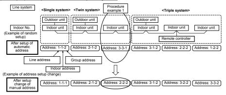
The above address is set by the automatic addressing when the power is turned on. However, line addresses and indoor addresses are set randomly. For this reason, change the setting to match line addresses with indoor addresses.
