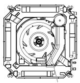
Be sure to remove the tape for transportation between the fan and the bell mouth.
